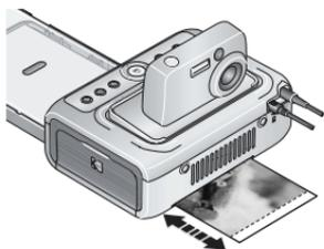
*The Print light blinks, and printing starts. The paper cycles four times before it is ejected. The first three passes apply layers of yellow, magenta, and cyan colors to the print, and the fourth pass applies the Kodak XtraLife coating that protects and preserves the image.*
