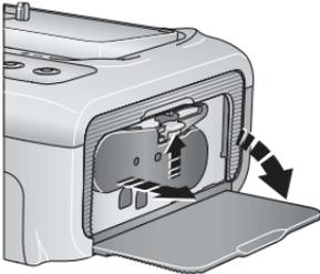
To remove the color cartridge, open the color cartridge door, then push up on the green lever and slide the cartridge out.
