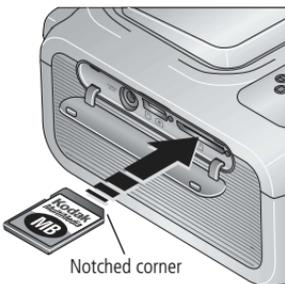
**2** Orient the card as shown, then push the card into the SD/MMC card slot to seat the connector.
